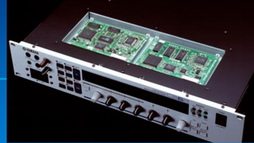
CS6R with top panel removed to show plug-in boards * On the CS6x, plug-in boards are installed from the bottom of the keyboard.
